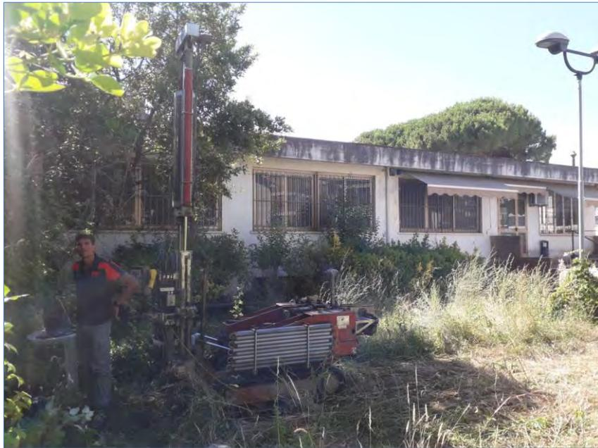
Figura 1: Prova penetrometrica CPTU P01
